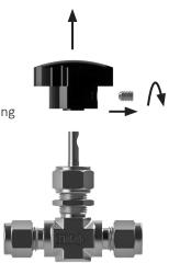
2. Use a wrench to remove the packing nut.
