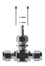
4. Turn the stem counter clockwise to remove the stem and packing from the body.
