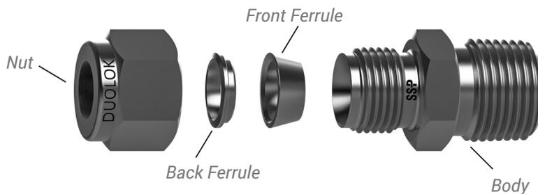
The double ferrule design, with the staged sequential swaging action of the ferrules during make-up, compensates for the variations in tubing materials, hardness, and thickness of the tube wall to provide leak-tight connections in an extensive range of applications.
