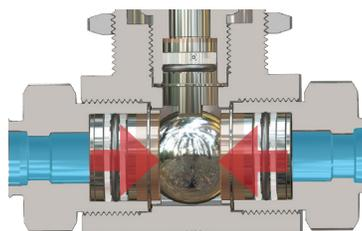
When the valve is open fluid flows through the valve (blue). Force from the springs (red arrows) applies pressure evenly to the seat gland, seat and ball.
