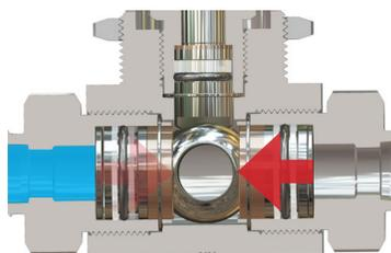
When the ball is closed under high pressure, the force of the upstream pressure forces the ball against the downstream seat to form a tight seal. Resistance from the downstream spring cushions the force of the ball against the seat to protect the seat and makes the valve easier to actuate.
