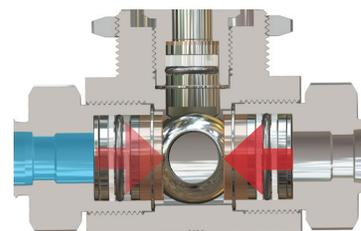
Under low pressure, there is much less upstream pressure on the ball and downstream seat. Without the mechanical force exerted by the seats and springs, the ball could disengage from the downstream seat.
