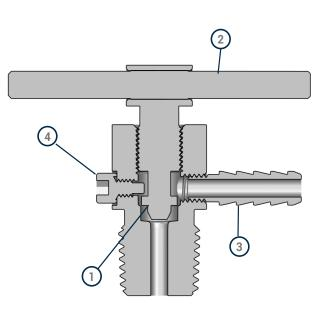
Warning! Bleed valves do not have stem packing. Therefore, operators may be exposed to system media that can escape during operation. Operators should open valves slowly with the vent port directed away from personnel and take appropriate precautions to protect themselve from system fluids.
