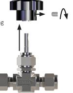
2. Use a wrench to remove the packing nut. (Make sure the packing springs are removed inside the packing nut.)
