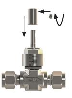
6. Place the handle over the sleeve. Use the 10-32 x 1/4" long set screw. Use a 3/32" Allen wrench to tighten the set screw until "snug" to secure the handle.
