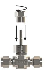
5. Place the sleeve over the stem. Use the 10-32 x 1/8" long set screw. Align the set screw hole in the sleeve with the drill point on the stem. Use a 3/32" Allen wrench to tighten the set screw until "snug" to secure the sleeve.
