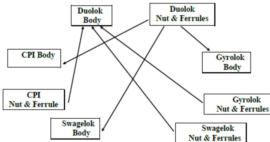
Figure 3.8.1, Interchange Test Combinations
