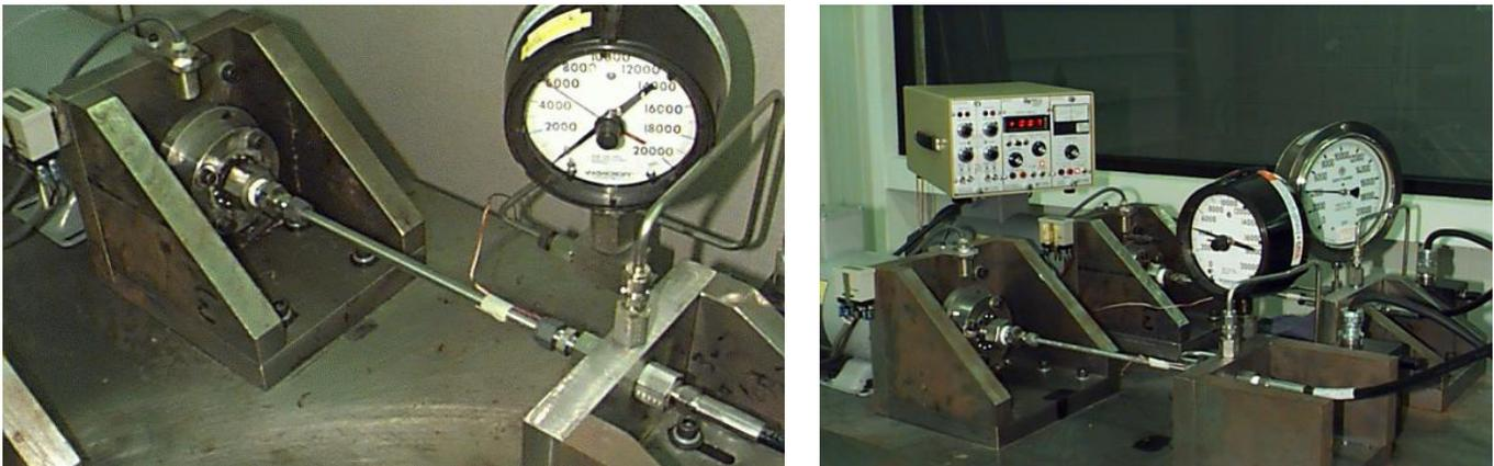
Figure 3.6.1 - 2, Vibration Test Stand and Test Configuration
