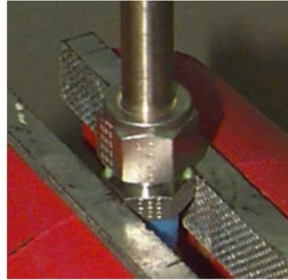
**Figure 2.1.2 Initial Makeup: Fitting Assembly**
