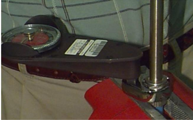
**Figure 2.1.1 Initial Makeup: Torque Measurement**
