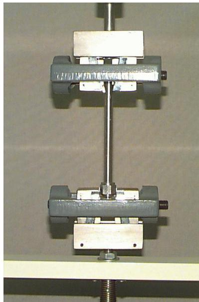
Figure 3.5.1, Tension Test Configuration.
