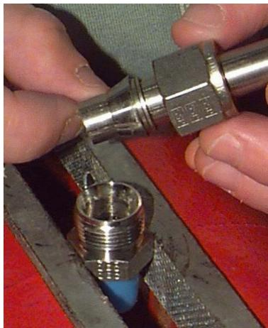
**Figure 3.4.1, Repeated Remake Test (Size 8 Duolok)**
