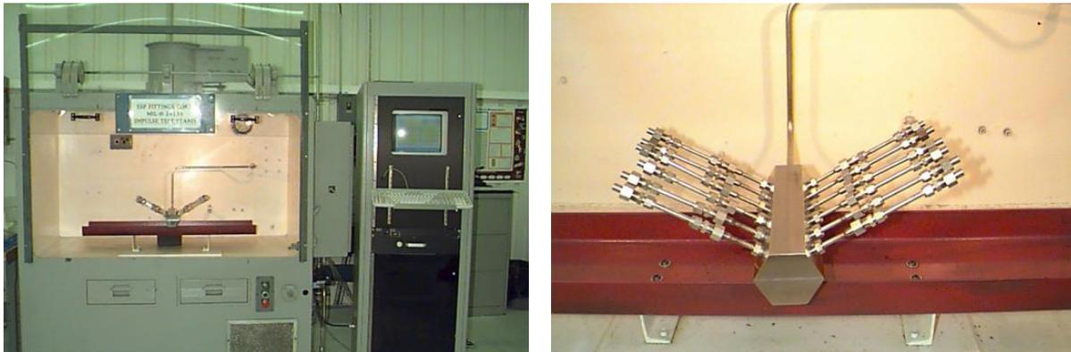
**Figure 3.3.1 - 2, Hydraulic Impulse Test Stand and Fixture**
