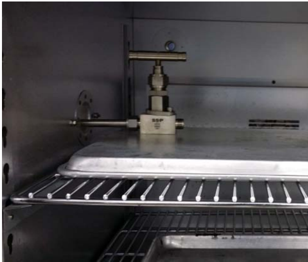
Figure 2.4.1 Leakage Test High Temperature Setup (200°F - 450°F)
