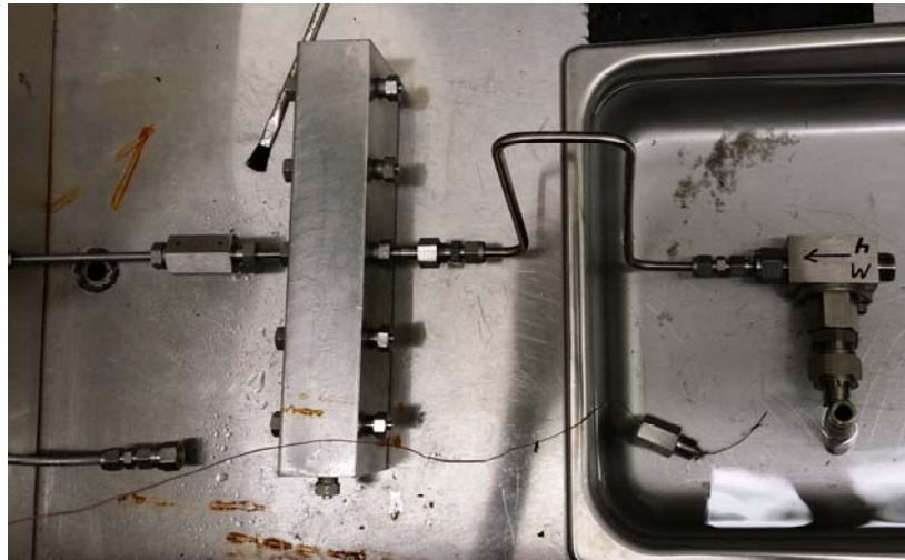
Figure 2.3 Leakage Test (Low Temperature) Setup
